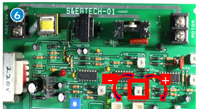
Set the Running Time. (Normally 5 sec.) (min.1 ~ max. 23 sec.)
