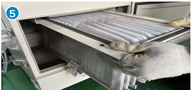
Carefully remove the filter as it is and discard as it is.
