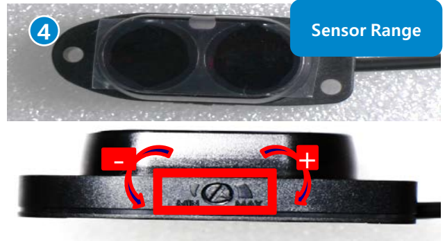
Set the Sensor Detection Range.
