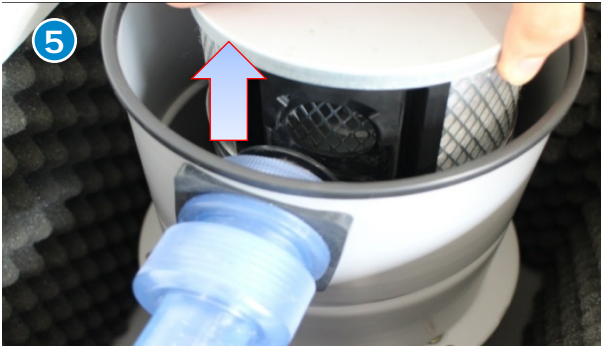
Detach the Filter by taking it up.
