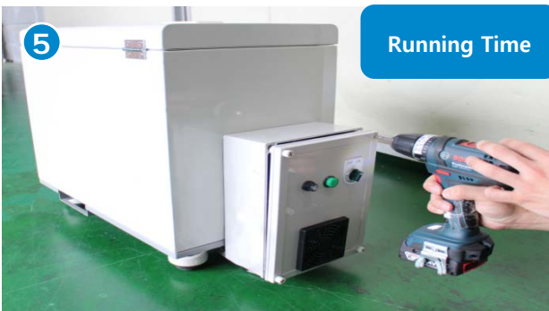
Running time is 5 mins. If you want to change, loosen 4 volts.
