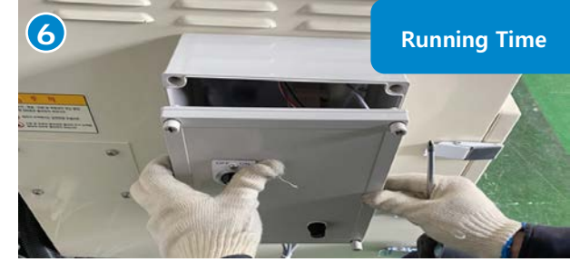
If you want to change the suction time, turn off the power and open the control box.
