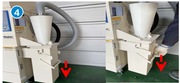
Make sure the cyclone dust tray is closed.
