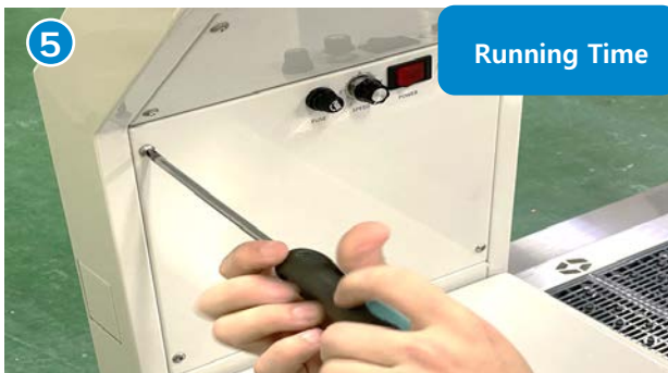
Set running time is 5 mins. If you want to change, loosen 4 volts.
