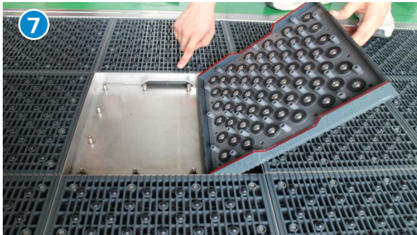
Match and place the red lines with the hole.
