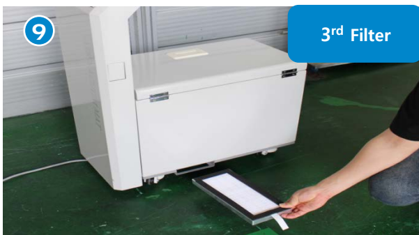
Exchange 3 rd filter with new one at the back of Dust Collector.
