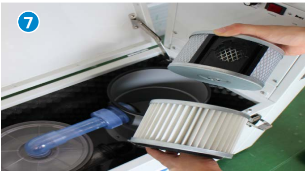
Exchange it with new one.
