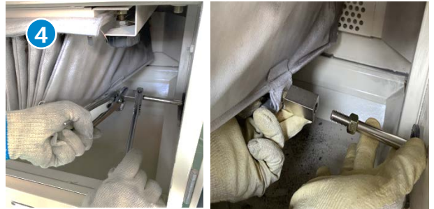
Separate the bolt and square bundle.
